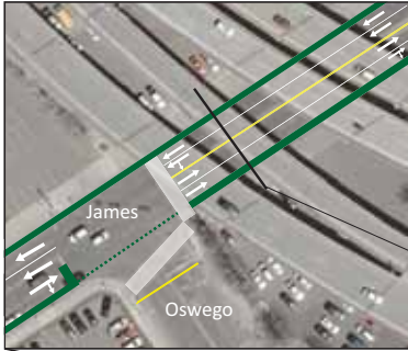
I-81 Overpass Connection (4 Lane to 3 Lane Shift)
